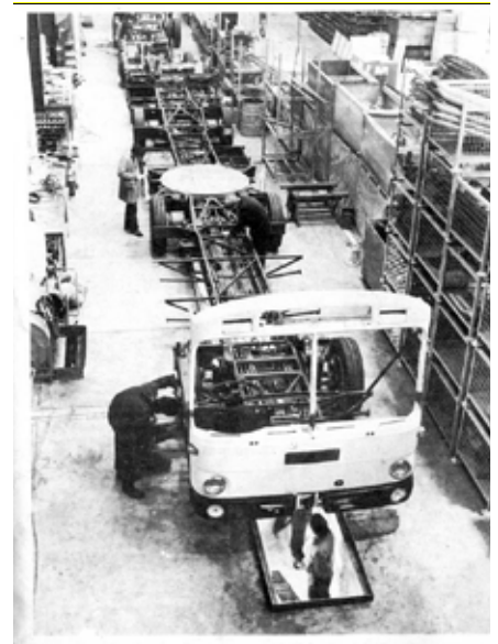
Figure 3.39 Assembling the chassis unit for the O-Bahn buses in the truck division at Mitsubishi Motors, 1983. Source: Three Diamonds , 1983, volume 2, number 3.
